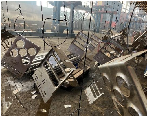
Figure 3: Enlarged loop formation of the wire suspension (left); Extraction process of the galvanized components (right).
