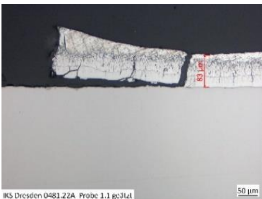
Figure 5: Micrographs: Missing zinc coating due to wire imprint (left); Touch-up with zinc dust paint. The edges are covered as required (right) [IKS Dresden].
