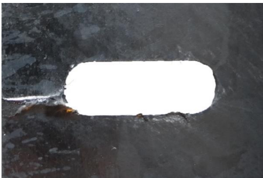
Figure 4: Zinc accumulation at the elongated hole due to the wire suspension (left) Detachment of the zinc layer due to dismantling (right).
