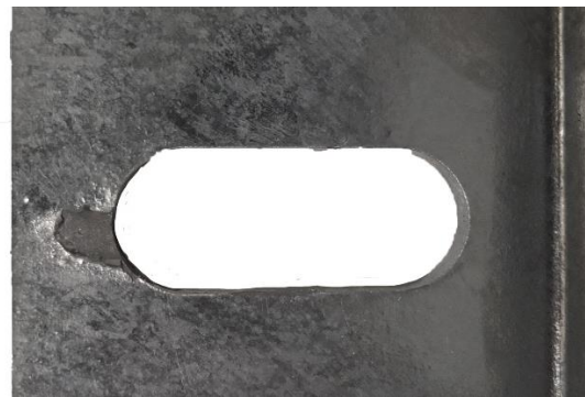
Figure 4: Zinc accumulation at the elongated hole due to the wire suspension (left) Detachment of the zinc layer due to dismantling (right).
