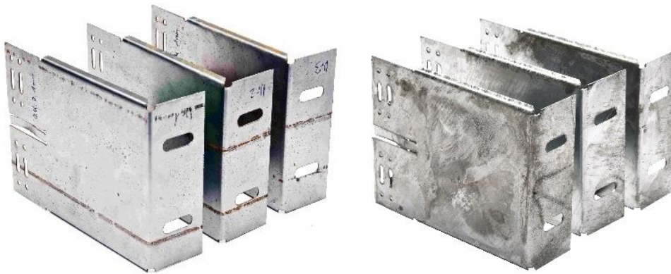
Figure 7: Excerpt of photo documentation: wall bracket variant 0; test series 1; t=1.00mm, steel 235, before galvanizing (left) after galvanizing (right).
